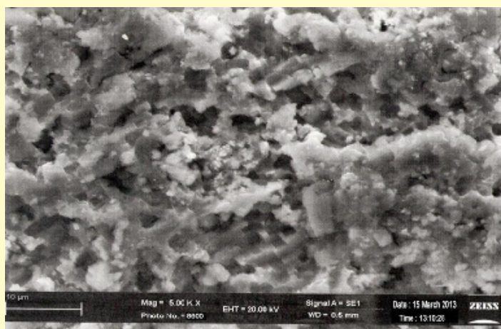
Figure 5.2: SEM (Magnified Image) of pure aluminium metal surface morphology immersed in 1.0N HCL for the period of 24 hrs.
