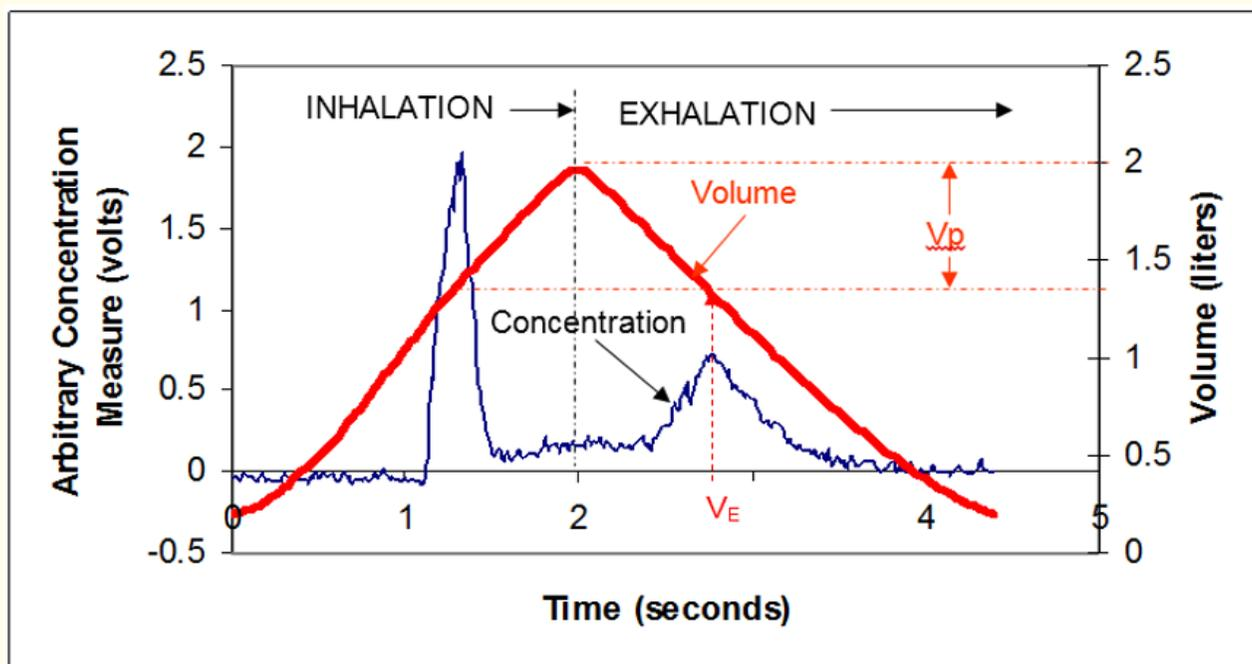
Figure 1: Test results from a 2.0 liter tidal volume maneuver with approximately a 0.6 liter (600 cc) volume of penetration ( $V_p$ ). As mentioned in figure 1,  $V_p = V_E$  and in this case  $V_E = V_M$ .
