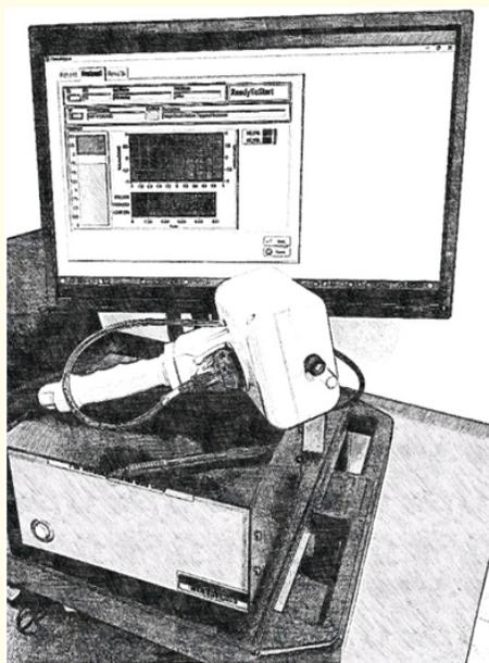
**Figure 3:** Aerosol Spirometer, consisting of a compressor (at base of picture) for the nebulizer and a handheld unit (on top of compressor) into which the subject can breathe while having both volume of air and aerosol concentration measured. The two piece unit (without the video screen, which was used primarily for initial training) is intended for home use.
