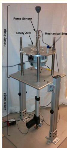
**Figure 1:** Overview of the haptic simulator.
