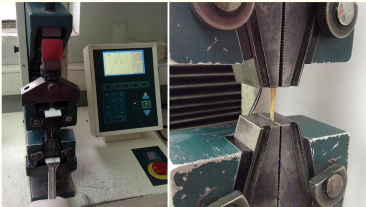
Figure 1: Tinius Olsen H5K-S® Universal Tensiometer (Serial No. 0138794) at a test speed of 5 millimeters per minute.
