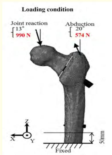
**Figure 2:** Load of hip contact force and gluteus medius with linearly increased magnitude up to cutout (if MAX 990N, 594N, respectively). Direction was constant.
