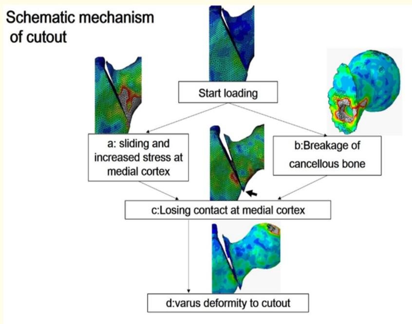
**Figure 3:** Mechanism of cutout under linearly increased loading: (a) sliding resulted in contact of medial cortex and elevated cortical stress followed by rotation; (b) cancellous bone breakage around the femoral neck; (c) loss of medial contact proved by declined stress (a black arrow); and (d) varus deformity leading to cutout after loss of medial sustaining.
