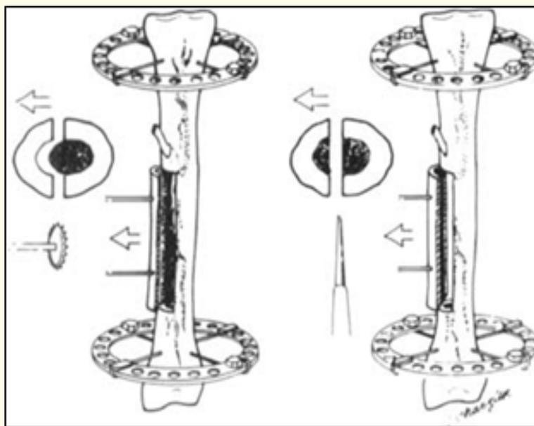
**Figure 4:** Ilizarov distraction osteogenesis in bone widening: osteotomy of the cortical segment, and the apparatus to displace the section of tibia1 cortex transversely [20] (with permission from the Wolters Kluwer Health).
