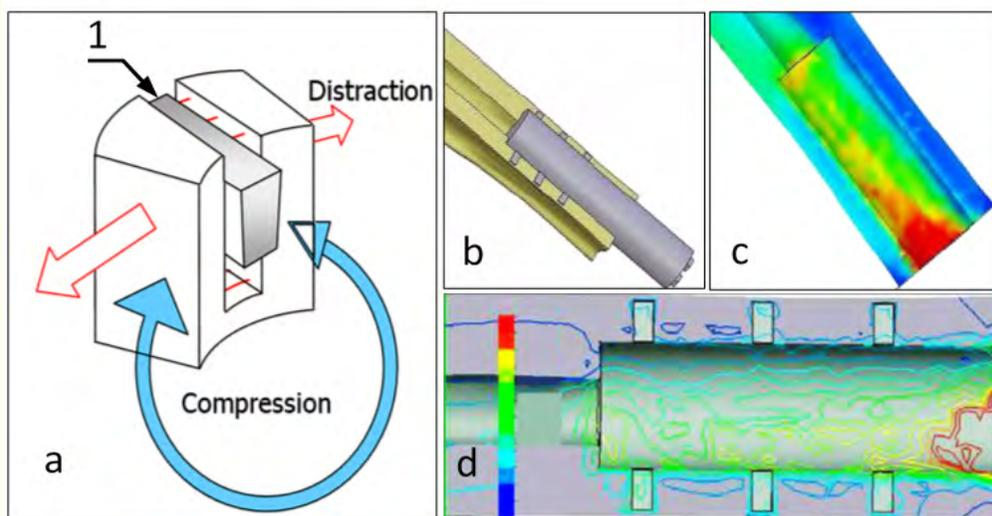
**Figure 2:** a: Press-fitting of fin 1 to slot in bone wall results in Ilizavov-type distraction (red arrows) and compression (blue arrow) due to elastic resistance of bone wall to widening [12]; b: 3-d CAD model of SBIP-F implanted in bone; c: Von Mises stress distribution in bone- pylon system for cylindrical SBIP; d: Von Mises stress distribution reduction in bone- SBIP-F compared to the SBIP without fins (c). Adopted from [25].
