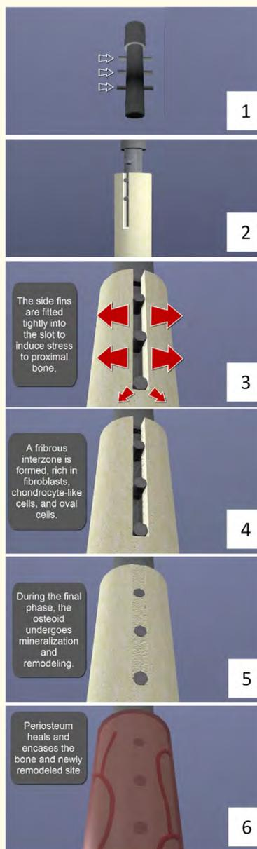
**Figure 3:** Illustration of the DI concept. Side fins of the stem are inserted tightly in the precut slots initiating distraction osteogenesis (Supplemental Video).
