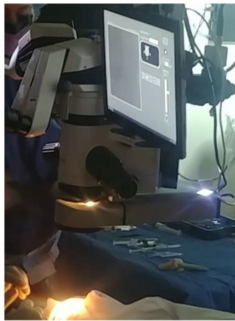
**Figure 1:** Polaris Keratoscope with tablet PC display, mounted on Leica M844 microscope (under microscope objective using dove tail adapter) during clinical tests at Pacific ClearVision Institute at Eugene, OR.
