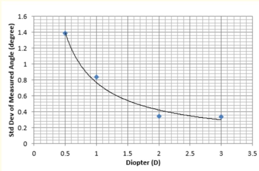
Figure 3: The dependence of astigmatism angle measurement accuracy of Polaris Keratoscope on the astigmatism value.
