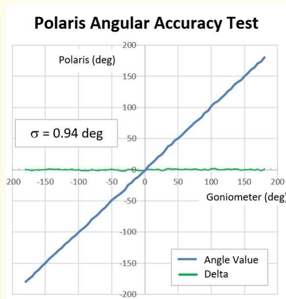
**Figure 2:** Polaris angular accuracy plot. Polaris angle measurements are plotted against goniometer angle values (45-degree line). The difference between two angle values is plotted as horizontal line. When statistical dispersion of the Polaris angular measurement is calculated it came to  $\sigma = 0.94 \text{ deg}$  - approximately 1 deg accuracy.
