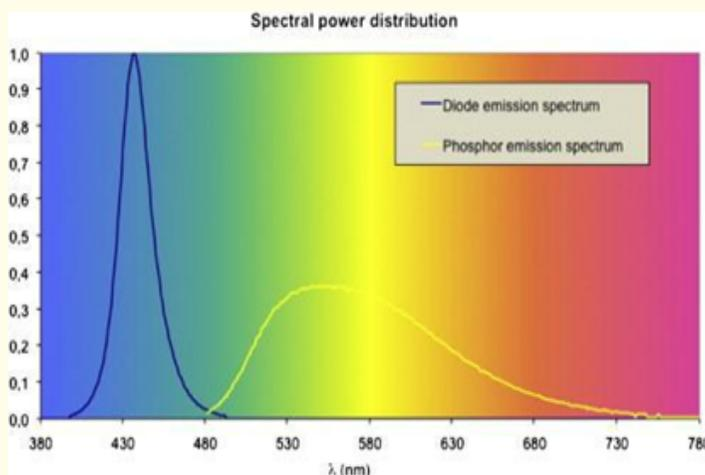
**Figure 1:** Spectral representations of using LEDs and with yellow secondary emission from phosphor, emitting with light. (www.sciencedirect.com, Behar-Cohen et al. (2011)) [4].
