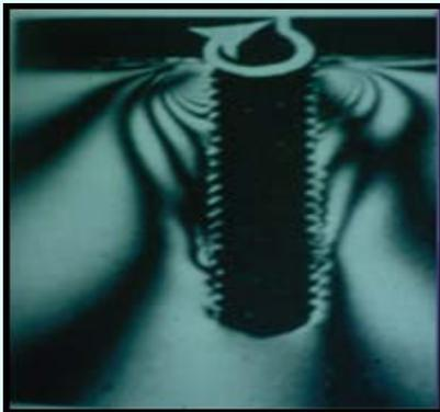
**Figure 1:** Three-dimensional finite element analysis of an implant under load in a bone model demonstrates the highest strain patterns are around the crestal 5 mm of an implant body [7].
