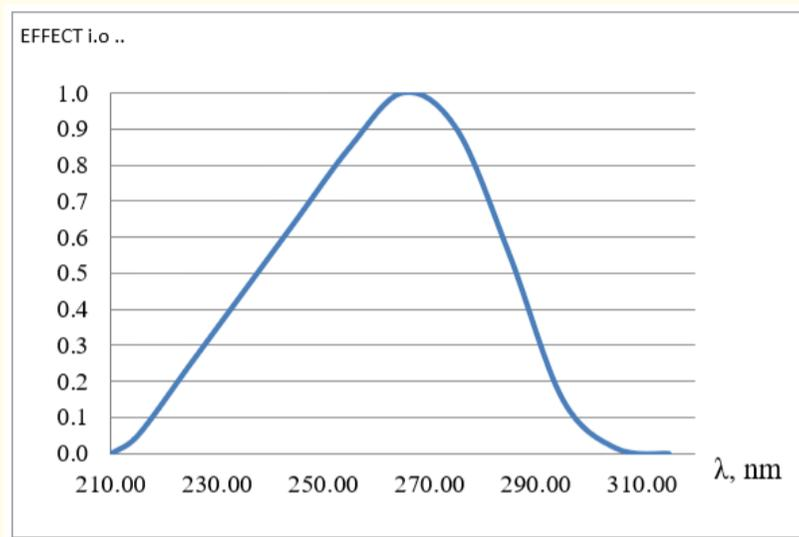
**Figure 1:** Curve of efficiency of bactericidal action of UV radiation.
