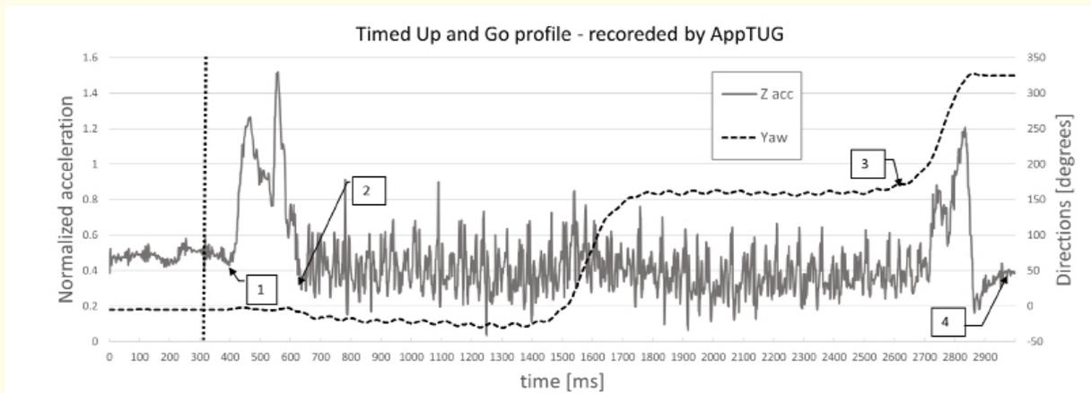
**Figure 1:** One accelerometer and one gyroscope as captured by AppTUG. The vertical dashed line indicates the Start signal. We can notice the stand-up time (SUT) between 1 and 2, each step in either direction, rotation circa 1.5 seconds, and sit-down time (SDT) between 3 and 4. Data is sampled at 100Hz, time is in milliseconds.
