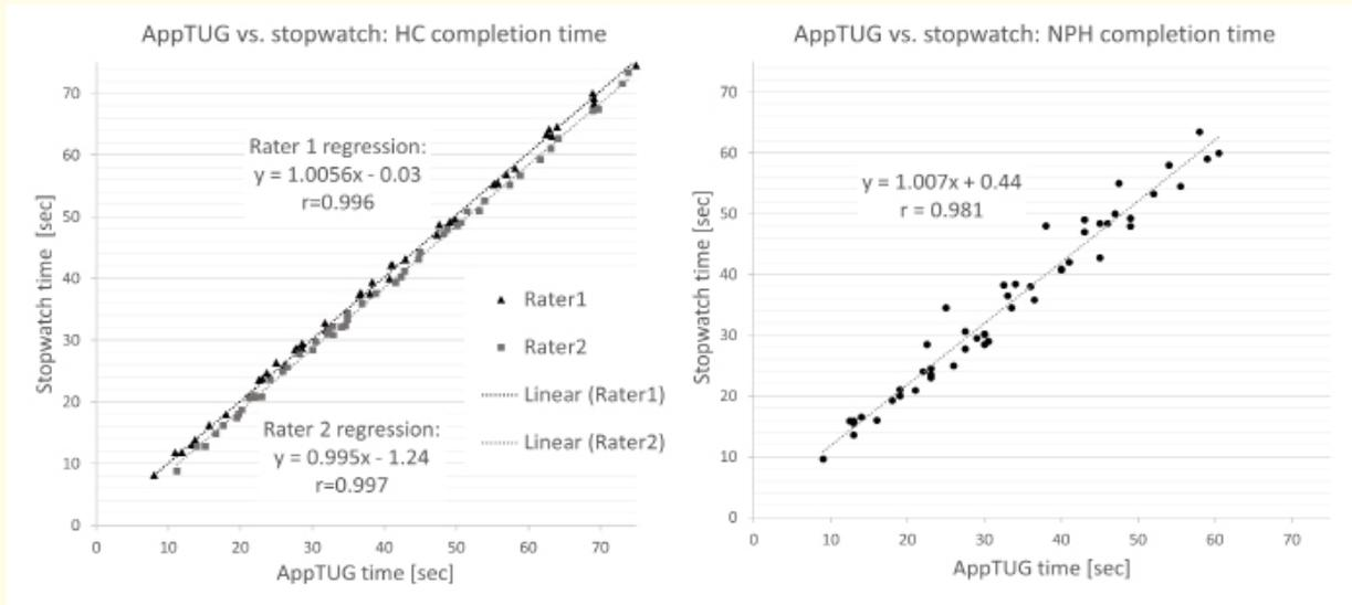
**Figure 2:** AppTUG measured time (X axis) and the time measured by an examiner using a stopwatch (Y axis) on NPH (left) and HC (right) subjects. Each graph consists of 50 results from the 25 NPH (left) and HC (right) subjects, one from the 3-meter and one from the 10-meter TUG for each subject.
