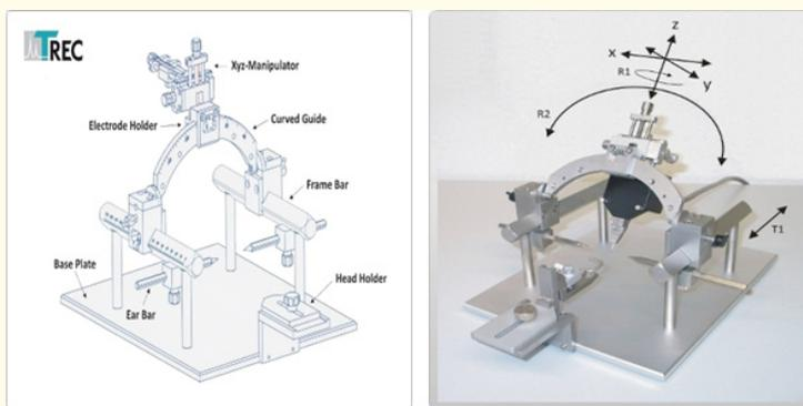
**Figure 3:** (left figure), The small animal stereotaxic instrument(SASI), an easy to be used instrument in small animals stereotaxic ,there is enough place for placement of cannula ,electrodes, and other devices. right Figure SASI has good degrees of freedom including: mouse adaptor , Head holders ,XYZ-Manipulator X,Y, Z adjustment, Rotation adjustment, and angle adjustment.
