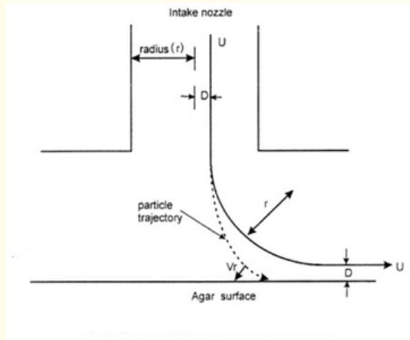
Figure 2: Principle of active air samplers and a petri dish.
