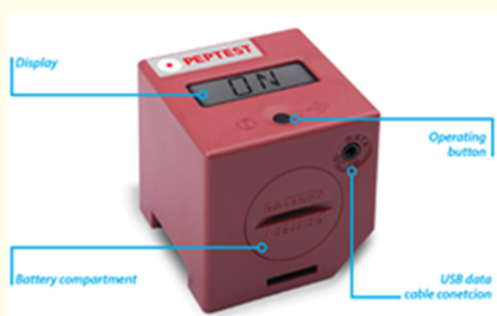
Figure 6: Peptest Cube reader designed to generate a pepsin concentration in ng\ ml^{-1} .
