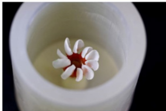
Figure 11: Waxed laminates lenses, ready for coating process, followed by wax evaporation process to continue with press injection of reinforced ceramic with lithium disilicate.
