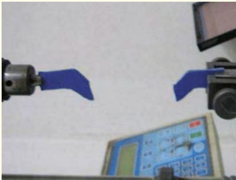
*Figure 11: Specimen after complete tearing.*
