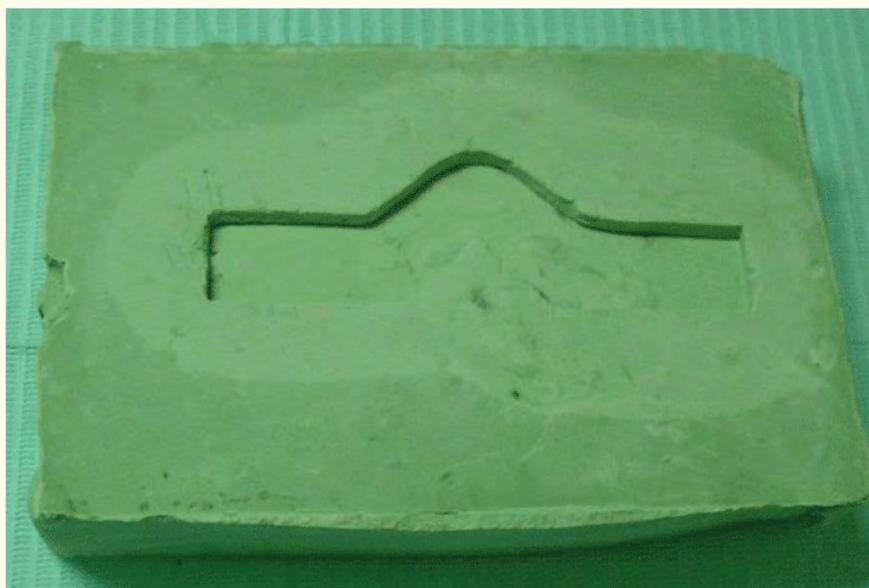
**Figure 6:** Un-nicked 90-degree angle shaped specimens according to American Society for Testing and Materials (ASTM) No.D624-911 for tear strength testing.
