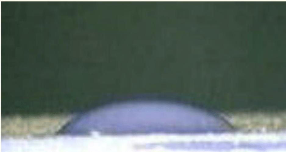
**Figure 14:** Captured photo for the wetting solution drop on the surface of horizontally-fixed VSE sample.
