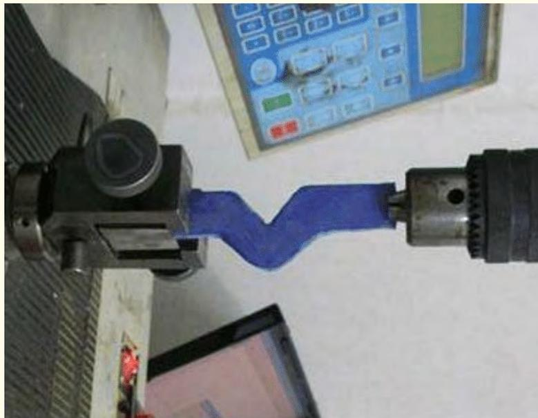
*Figure 10: Tear strength testing of vinylsiloxanether.*
