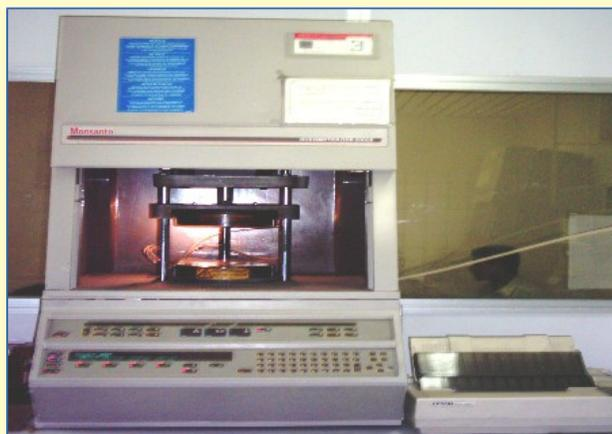
**Figure 1:** Oscillating disc Rheometer.
