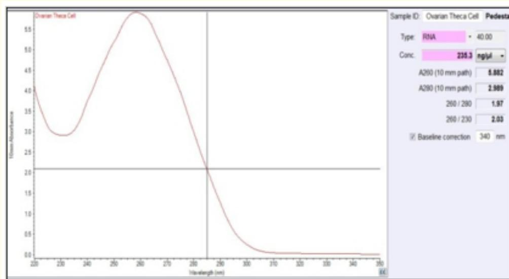
**Figure 3:** Measuring the concentration and assessing purity of RNA using NanoDrop spectrophotometer.
