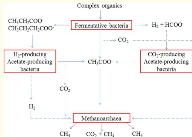
Figure 1: Methanogenesis in anaerobic environments (Robert 2001).
