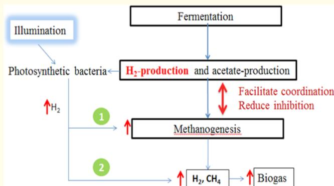
**Figure 2:** Pathway of the effect of illumination on biogas yield.
