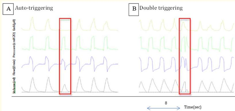
**Figure 2:** Auto-triggering and double triggering.
