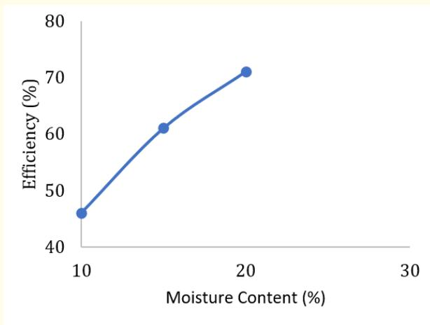
Figure 2: Effect of moisture content (dry basis) on efficiency.
