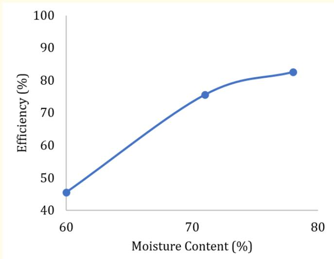
Figure 1: Effect of moisture content (wet basis) on efficiency.
