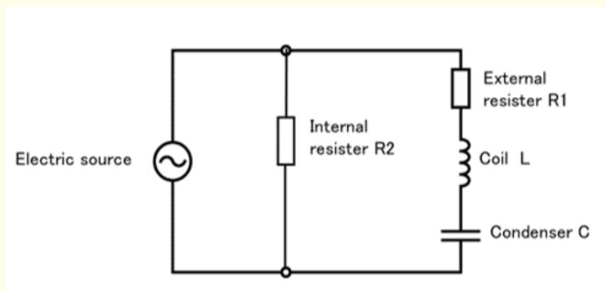
**Figure 2:** Basic RLC circuit (resistor, inductance and condenser C).
