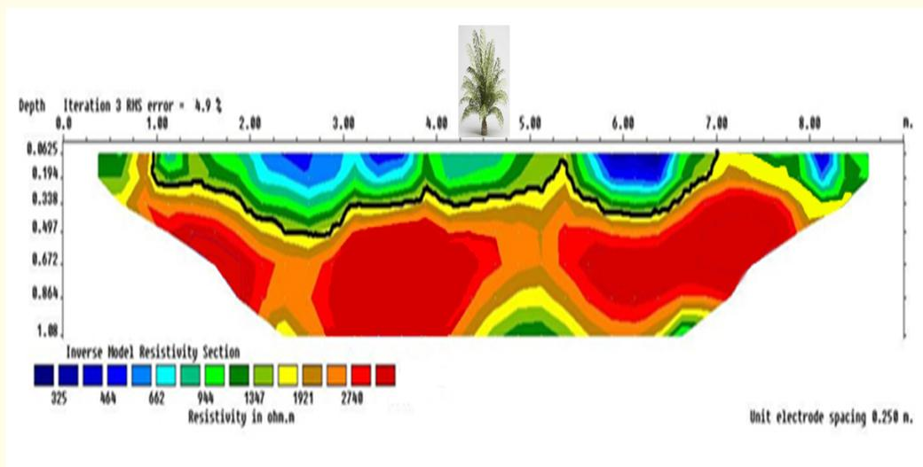
Figure 1: 2D Resistivity of Cross Section of Track I.
