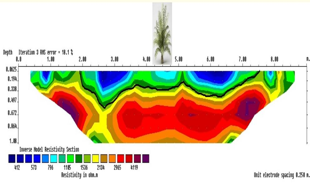
**Figure 2:** 2D Resistivity of Cross Section of Track II.
