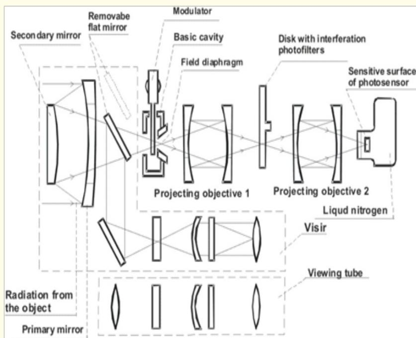
**Figure 1:** The optical scheme of OMS "SimAr-A" complex.
