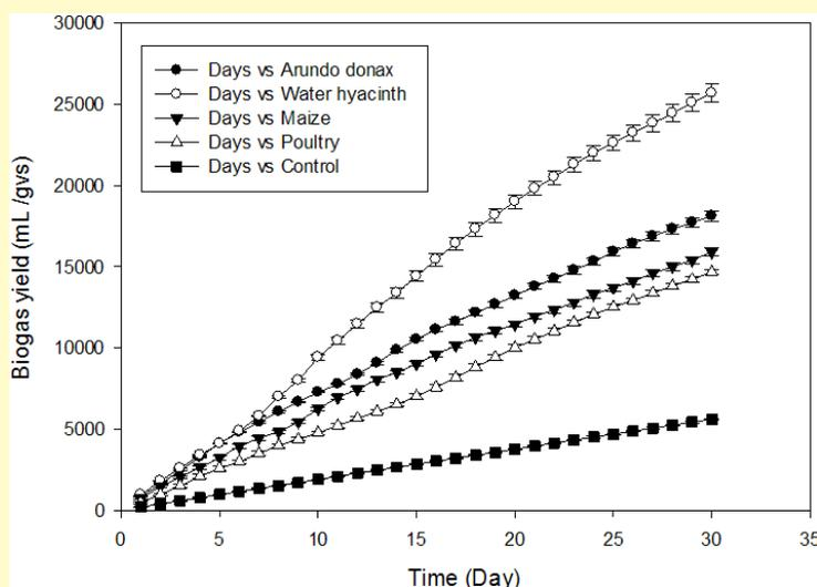
**Figure 3:** Cumulative biogas generation from mono-digestion of water hyacinth, maize, giant reed, poultry waste and Control.
