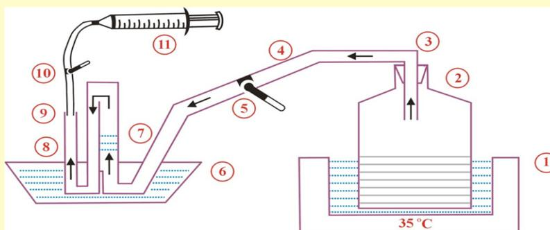
**Figure 1:** Experimental set up, 1. Thermostat 2. Bioreactor 3. Rubber bung 4. Gas pipe from reactor to graduated cylinder, 5. Valve from reactor to Gas collector (500 ml), 6. Acidified water, 7. Gas collector, 8. Bucket containing Graduated cylinder (500 ml), 9. Removal pipe for Biogas 10. Valve in the removal pipe, 11. Syringe 60 ml.
